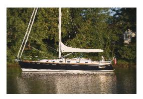
We motored south into Biscayne Bay before hoisting the mainsail. The main in the tall Cruise Control Rig sits in a pocket boom that is wide enough for the full battened sail to flake itself and then get covered with a nifty sail cover. The mainsheet and halyard run aft to a cabin top winch next to the companionway, so hoisting the sail and then trimming it is simple.
